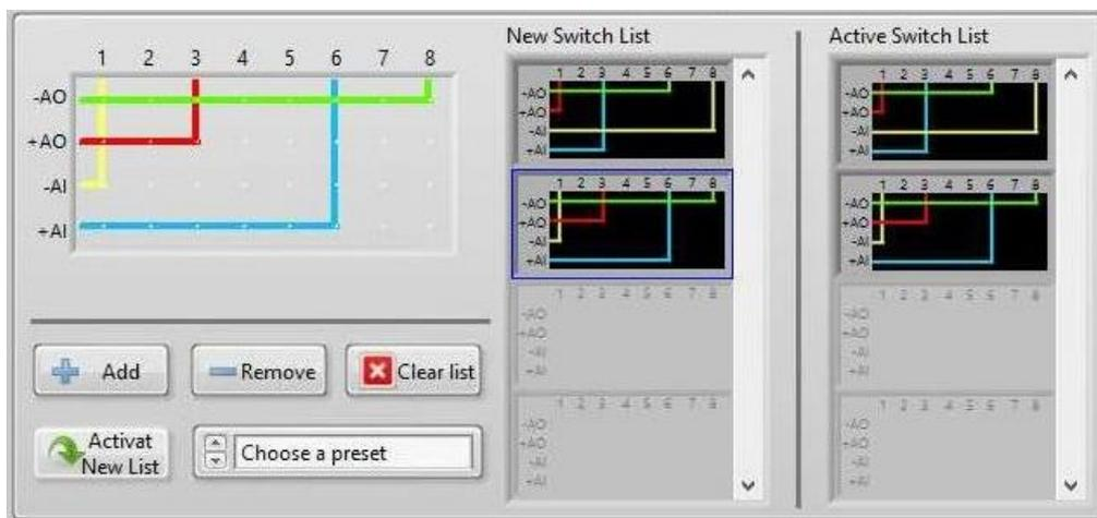
With the Add and Remove buttons, a New Switch List can be built up step by step, which is then transferred to the device using the Activate New List.
